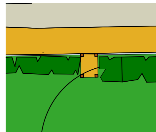
3. Cut back hedge to form 1.2m wide entrance. Install timber edging and gravel and timber posts to mark position of entrance.
